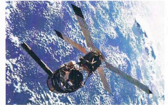
Skylab’s orbit decayed faster than expected because greater than expected activity on the Sun “puffed up” the top of Earth’s atmosphere, slowing the station down. Skylab was destroyed as it burned up in the atmosphere in 1979.
