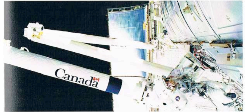
Canada’s Space Station Remote Manipulator System can creep slowly along the outside of the space station like an inchworm.
