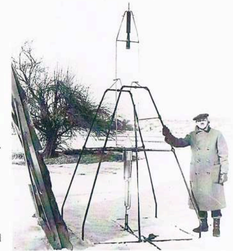
Dr. Robert H. Goddard standing next to the rocket that would make the world's first liquid propellant rocket flight on March 16, 1926.
