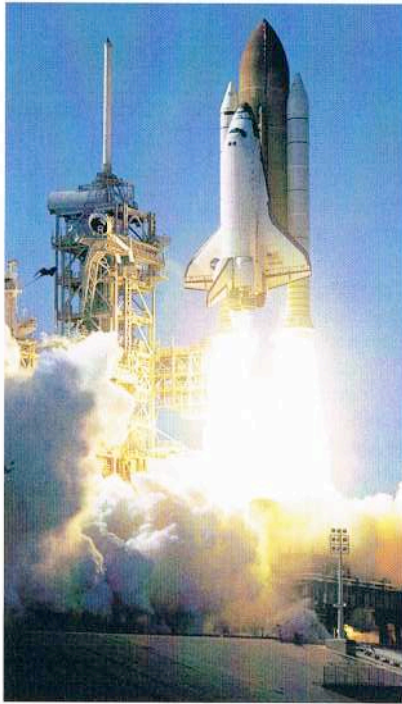
A combined thrust of almost 7.8 million pounds starts the shuttle on its upward climb. Brilliant orange flames shoot out the back of the boosters and stretch downward for 600 to 700 feet—more than three times the length of the vehicle itself.
